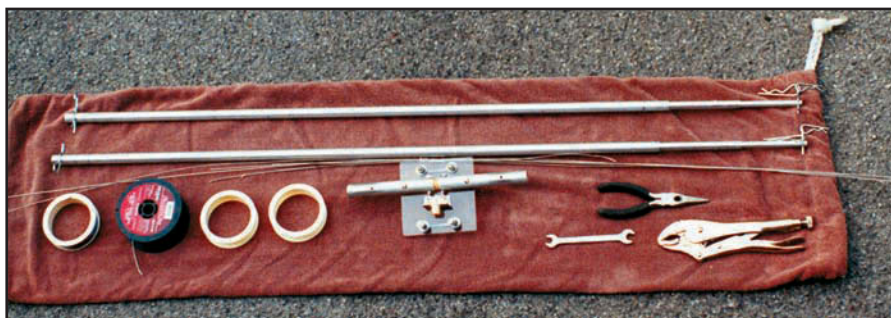
Figure 8—The entire inverted-U antenna parts collection in semi-nested form, with its carrying bag and the three dedicated tools for field assembly and disassembly.
